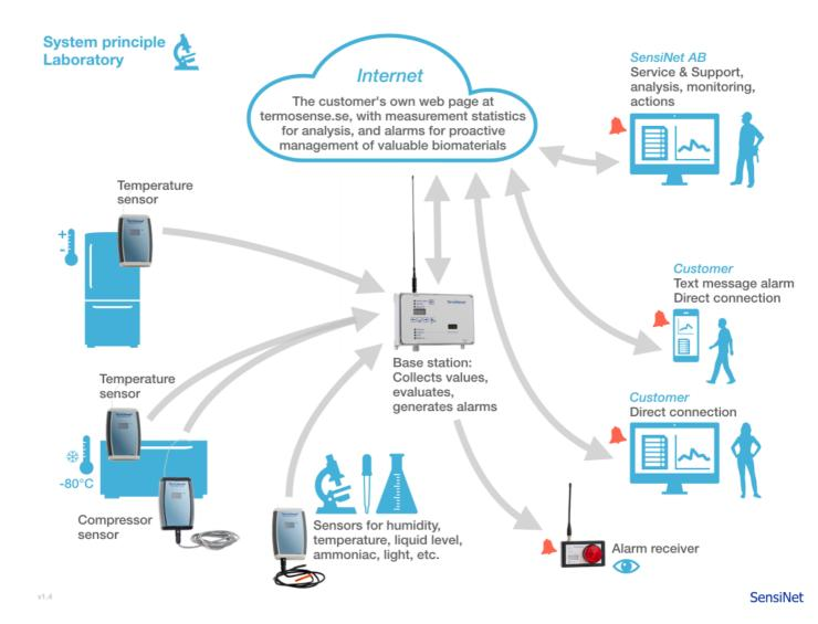
The wireless sensors form the basis of the TermoSense® system. They are tight, durable and maintenance-free with up to 17 years of battery life.
